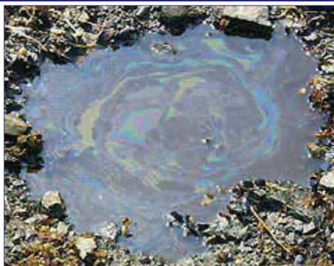
Motor oil and other oil-based chemicals can be recognized by a characteristic rainbow-colored sheen
